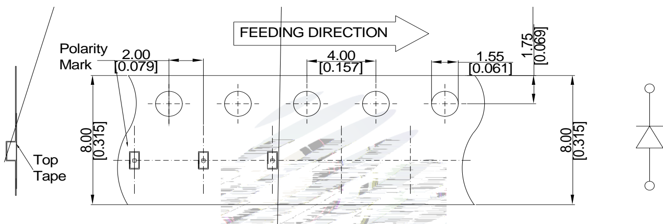
Fig.2-1 Carrier Tape Dimension 载带尺寸
