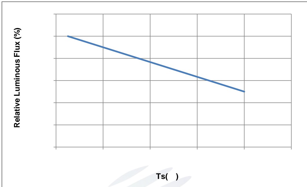
Fig. 1-9 Solder Temperature Vs Relative Intensity
